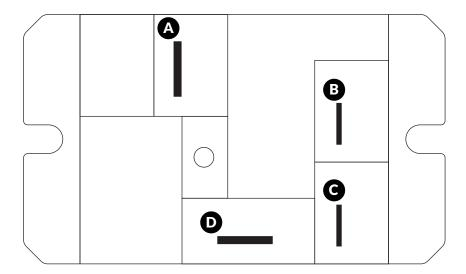
**Terminal** Connection A ■ AC (L) **OUT** AC device Line L B BRNKL connector Slot **2 3** yellow 0 12V DC constant power, fuse-protected 🕀 red 0 AC (L) IN AC source Line L
