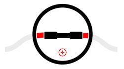
2. Connect and crimp the **black**  $\bigcirc$  wire and the black  $\bigcirc$  power lead with a heat-shrink butt connector.
