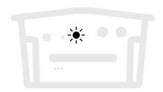
> If the light is **flashing**, the satellite device isn't connected. Check the cable connection. then repeat the test.
