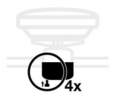
Before tightening the screws, align the sides of the device with the horizon.
