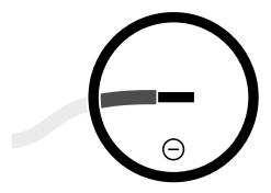
3. Connect and crimp a ring terminal to the wire.
