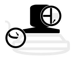
2. Attach the mount using the supplied 12 mm hex screws, metal washers, and plastic washers.
