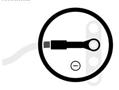
2. Secure the wire with cable ties and mounts.
