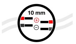
3.. Connect and crimp the red wire and the red  $\oplus$  power lead with a heat-shrink butt connector.
