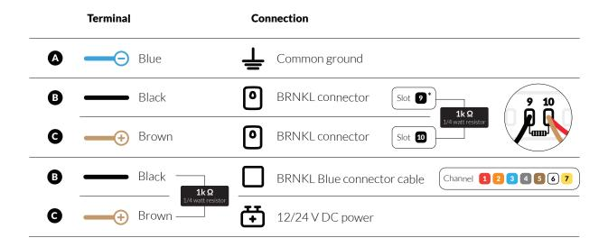
\* Connect a shore power sensor to an alternate BRNKL connector slot. See Shore Power Connections for details.
