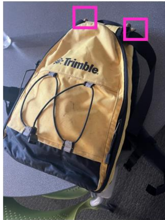
Make sure to have your Trimble backpack with you. Attach R2 to one of the attachments at the top. R2 needs to be upright and uncovered to work.
