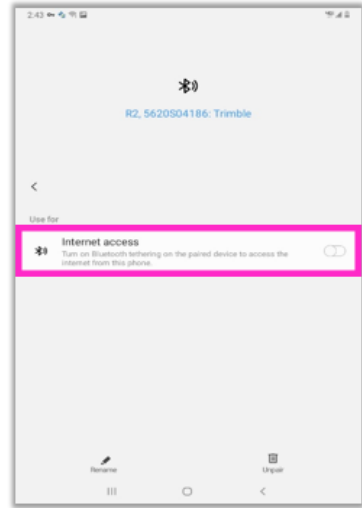
Make sure bluetooth is not being used for internet access by turning internet access off.
