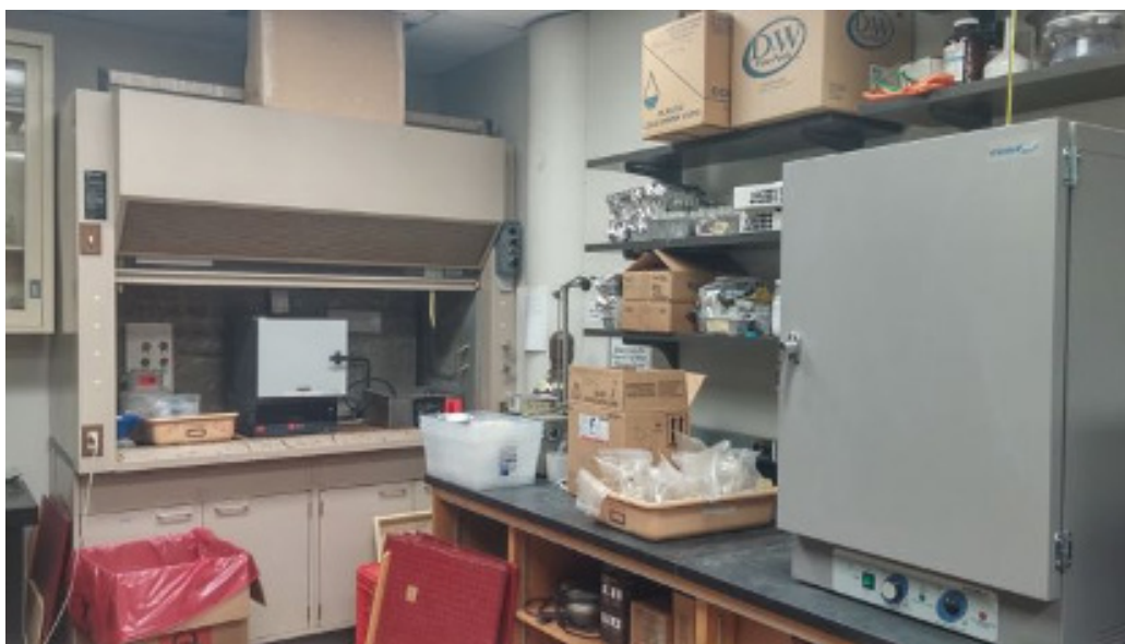
Equipment in Dr. Katalin Szlavecz's soil lab at the Johns Hopkins University Homewood Campus. The furnace is the white door below the fume hood in the background. The drying oven is the large gray box in the foreground.
