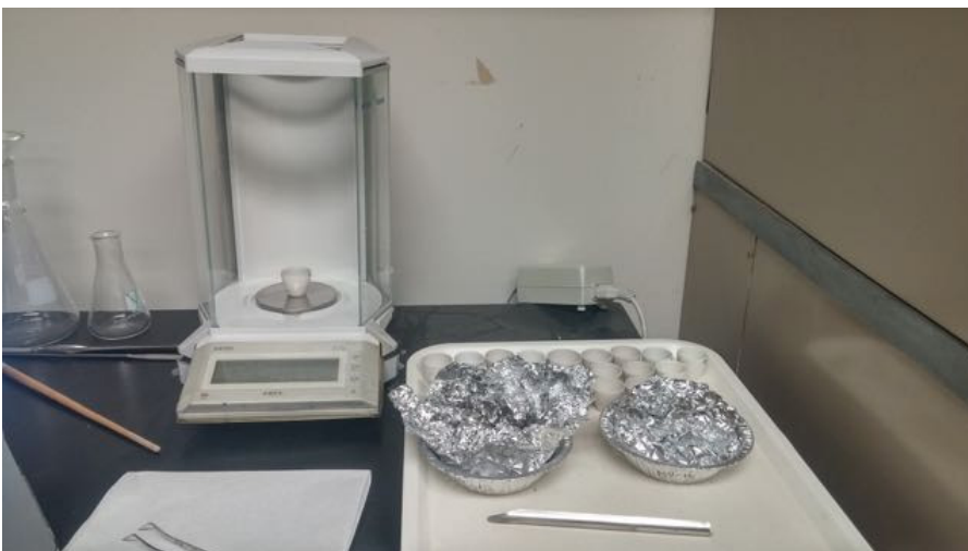
Weighing organic matter samples and crucibles in the analytical balance.
