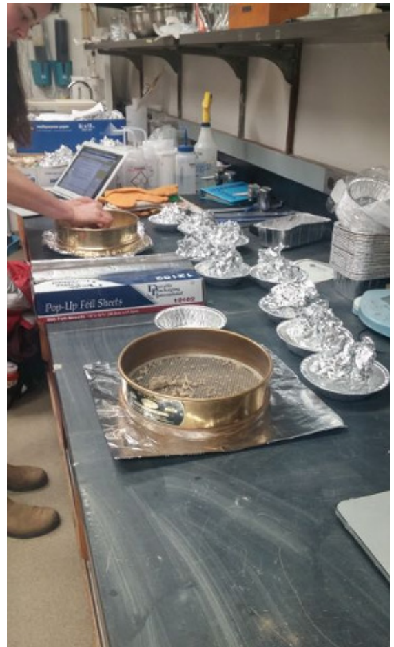
A lab bench set up is shown on the right. Each sample from the site is contained in the aluminum foil and trays, and samples are organized numerically. In the foreground, a 2-mm sieve sits on a sheet of aluminum foil. Any materials too large to fit through the sieve are transferred to the aluminum tray for weighing.
