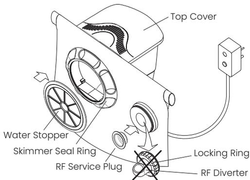
c. Detach the Locking Ring and RF Diverter by turning it counterclockwise. Insert the Service Plug.
