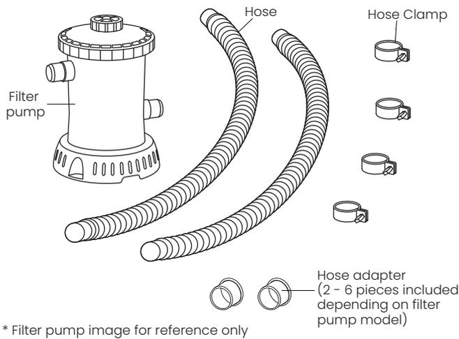
2. Add a Hose Clamp on each end of the hose. Insert a Hose Adapter to one end of the hose and then, connect the hose to the Filter Pump Inlet.
