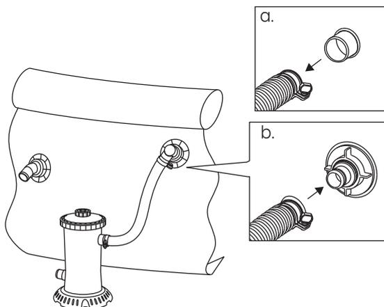
4. Tighten the Hose Clamps to prevent loosening and water leakage. Repeat steps 2, 3 & 4. Connect the Return Fitting to the Filter Pump Outlet (sequence as shown below).
