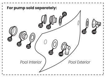
3. Install the Return Fitting @ on the Inlet opening of the pool.
