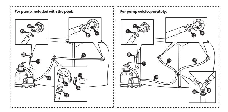
17. Make sure the Hose Clamps (5) seal tightly over both the Hose (5) and O-Rings (8). Tighten all the Clamps with a cross-head screwdriver (not included).
