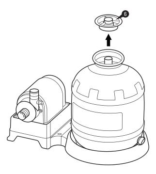
8. Install the 6-Port Valve 10 to the Sand Tank 2, and ensure if fits securely into the Center Pipe 5. Rotate the Valve so that the triangular mark under the Pressure Gauge 20 is aligned with the triangular mark on the Sand Tank 2.
