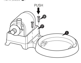
3. With the Drain Valve of the Sand Tank 2 pointing outwards, place the Sand Tank 2 onto the Sand Tank Base 1.
