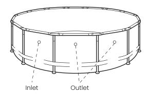
2. Install the Suction Fitting components into the Outlet opening.
