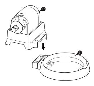
2. Insert and push the Lock Pins (3) all the way down to secure the Pump (7) to the Sand Tank Base (1).
