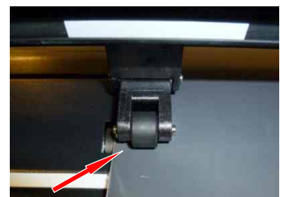
Left Pinch Roller in Correct Position
