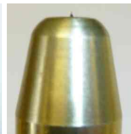
Correct Depth for ThermoFlex or Sign Vinyl
