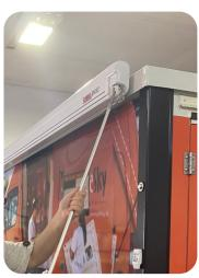
As the awning approaches full extension, it is now time to unhook the two supporting legs. First, the legs must be grasped near their hinge-point and pulled toward you. They will now be able to be rotated downward and extended to the marked position. Please ensure the securing knob is sufficiently tight.
