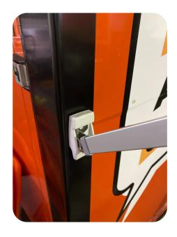
The awning may now be readjusted using the crank handle to ensure the shade sail is sufficiently tight.
