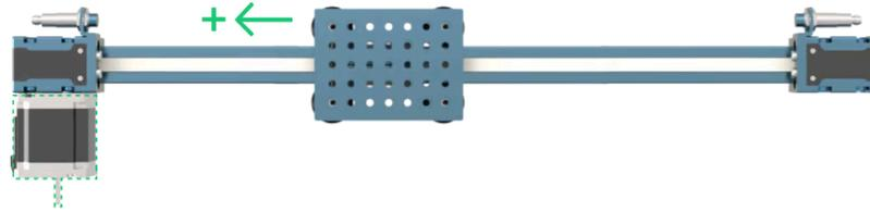
Figure 12: Axis direction based on motor location
