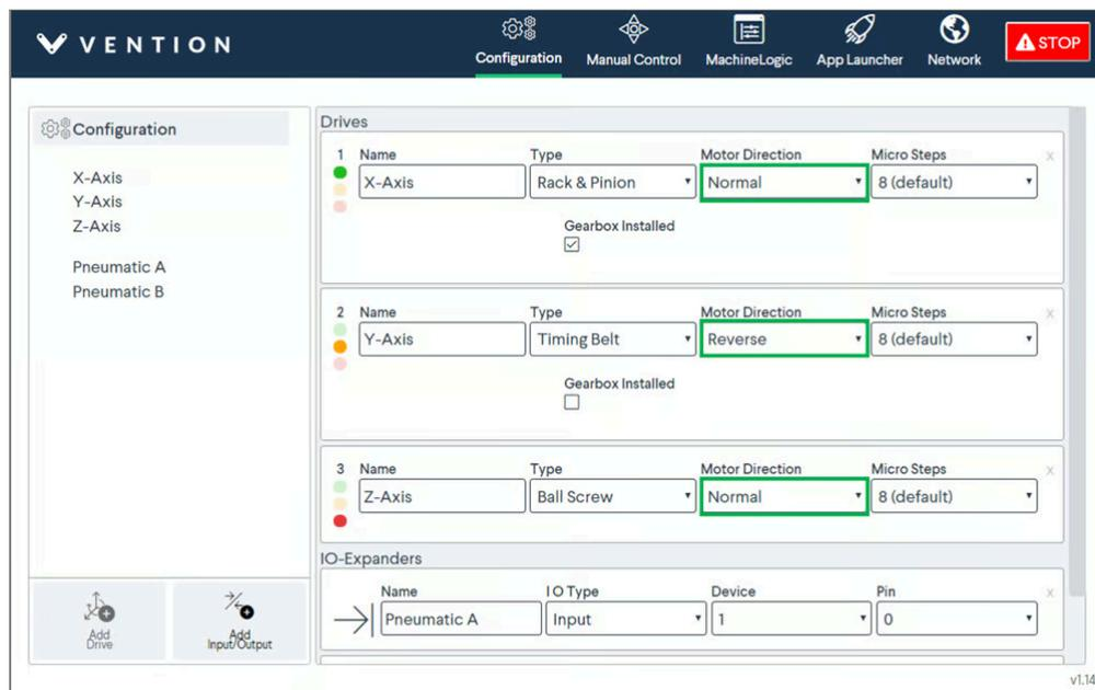
Figure 14: Axis direction reversal
