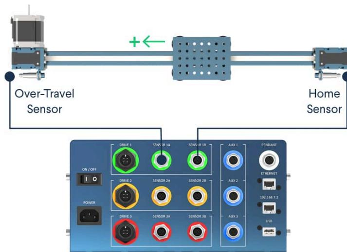
Figure 15: End-of-travel sensors connection in reversed mode
