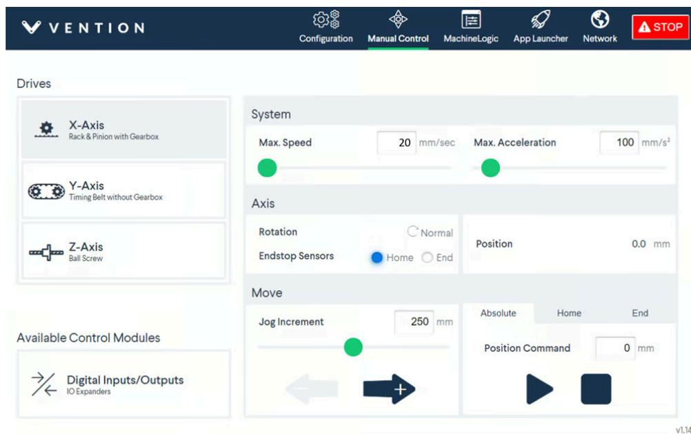
Figure 17: Setting max. speed and max. acceleration
