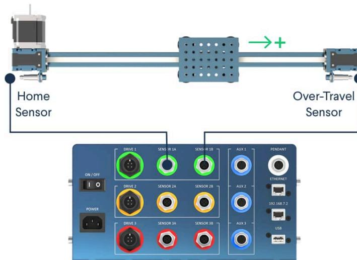
Figure 13: End-of-travel sensors connection
