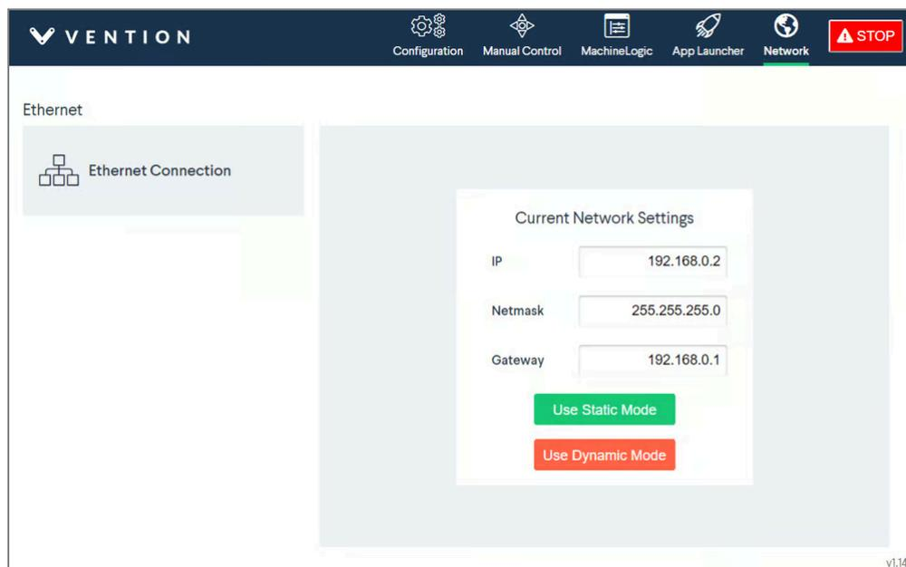
Figure 8: MachineMotion network settings
