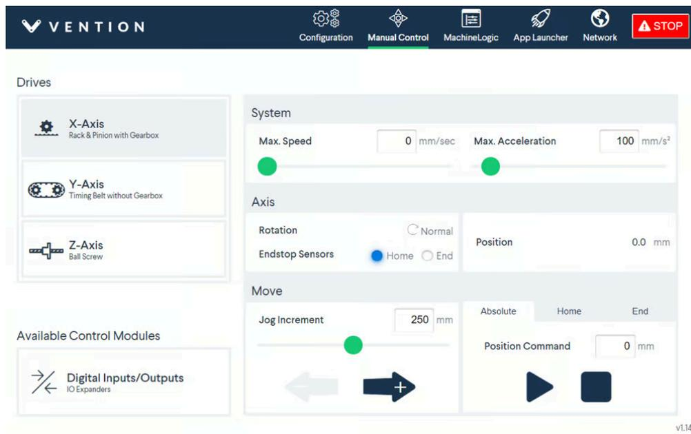
Figure 18: Triggering the home sensor
