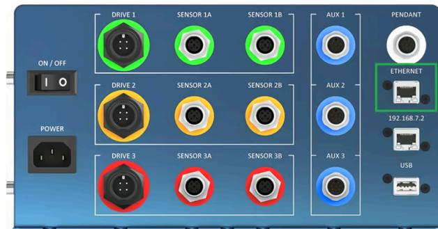
Figure 5: The standard configurable Ethernet connector.
