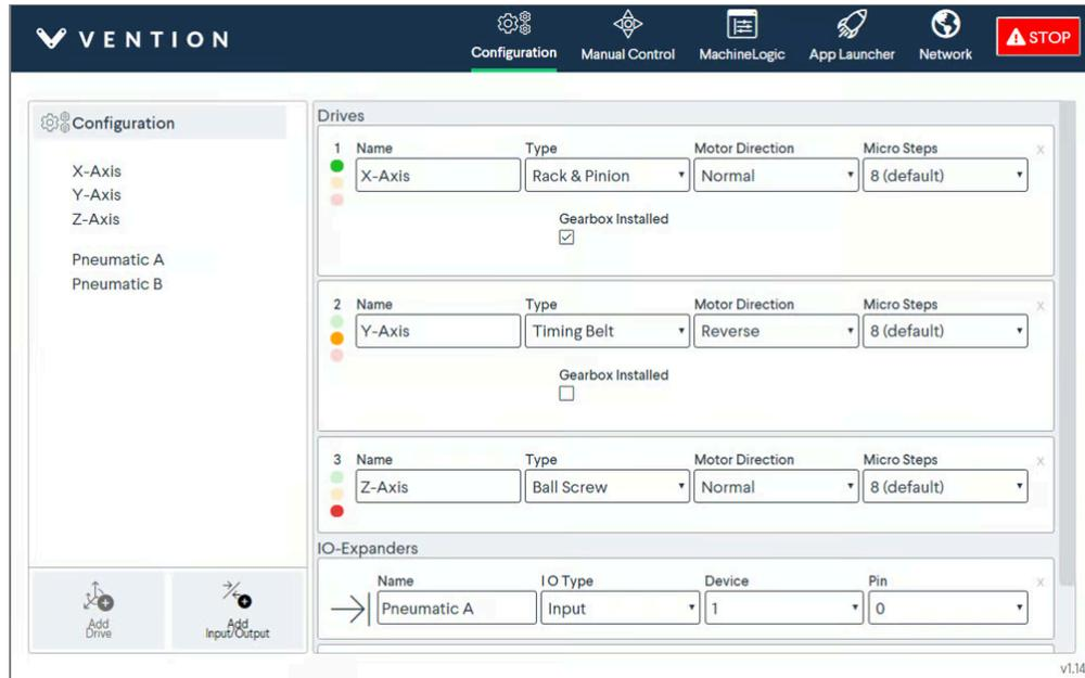
Figure 9: Control Center axis configuration tab
