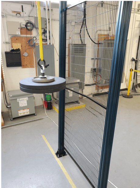
Post-impact deformation of machine guarding panel
