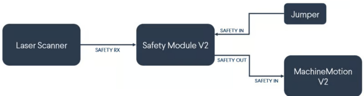
Safety Module with laser scanner (no muting)
