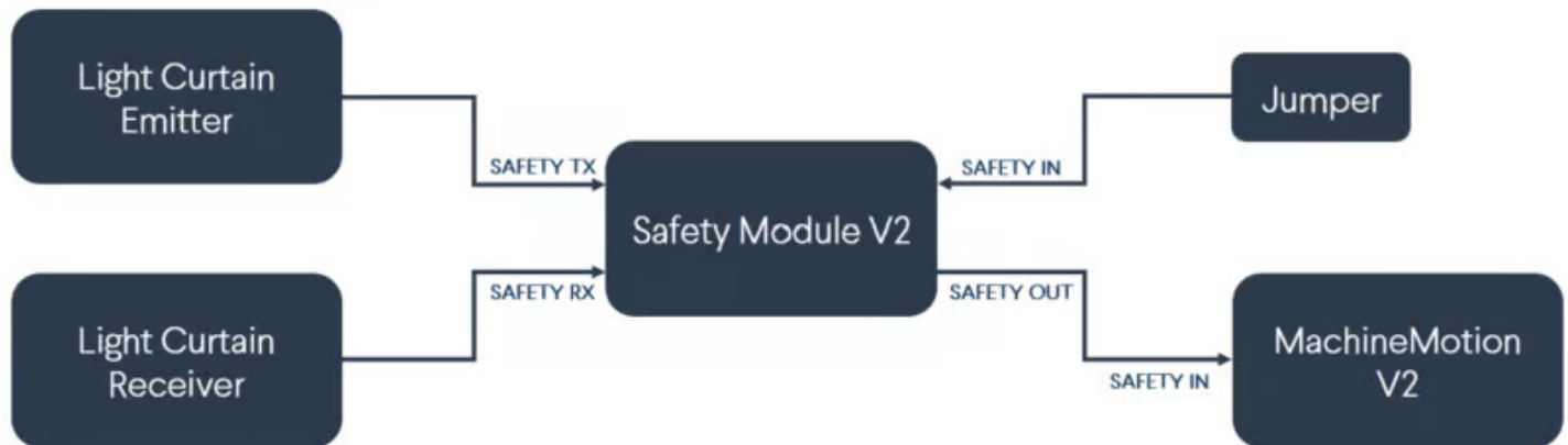
Safety Module with light curtains (no muting)
