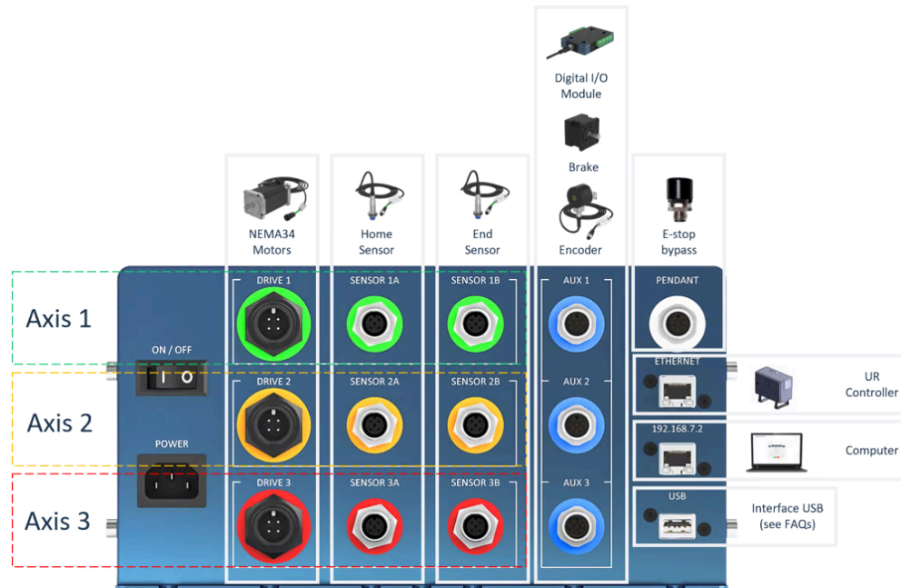
Figure 5: Example MachineMotion system with Ethernet peer-to-peer connection to a UR controller
