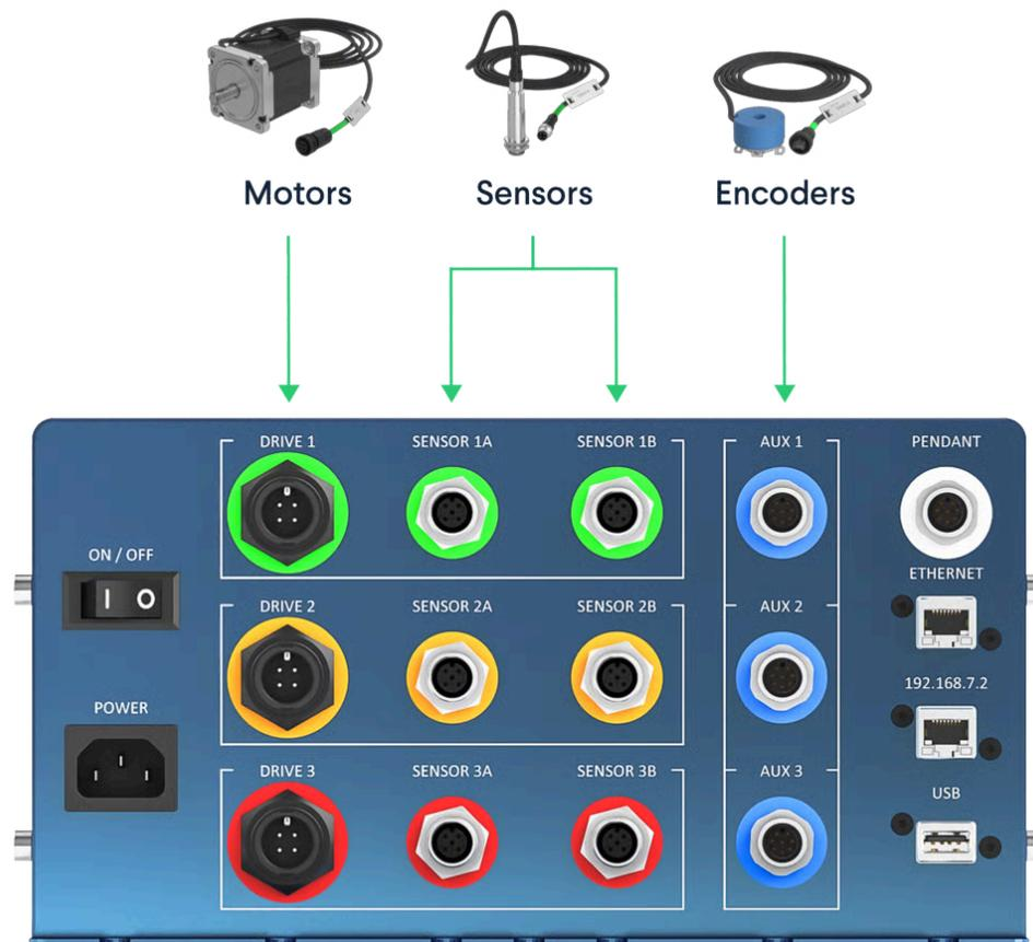
Figure 9: Connection ports for the MachineMotion Linear Axis Range Extender
