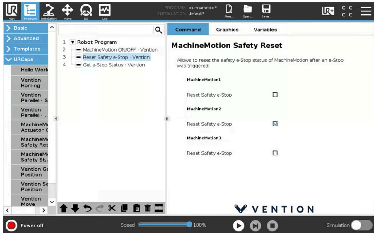
Figure 23: Vention URCap safety reset details
