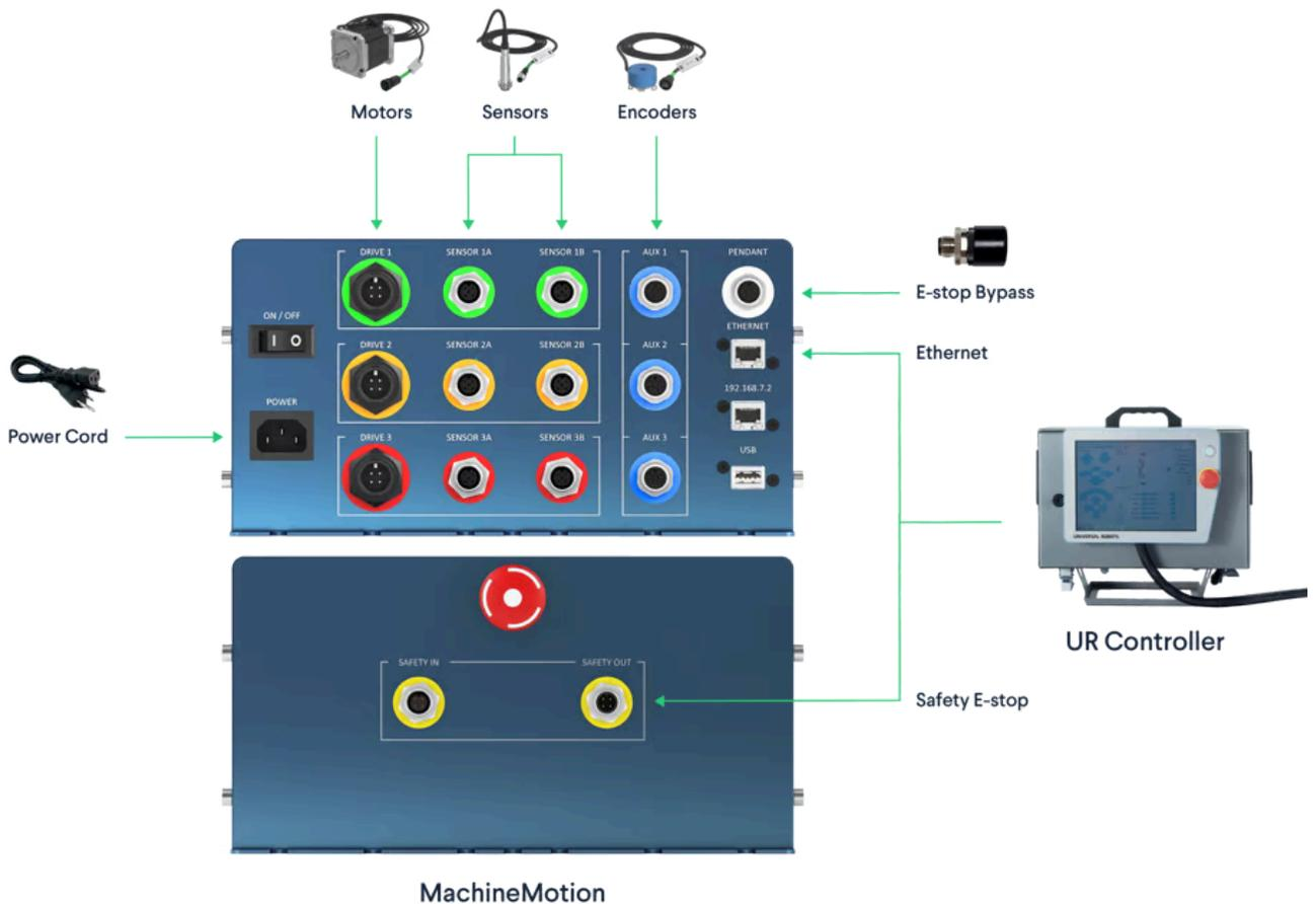
Figure 7: MachineMotion-to-UR controller connections
