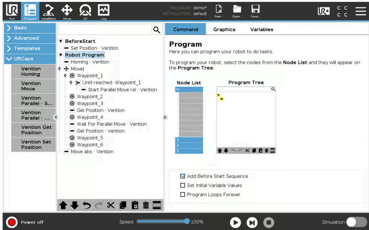
Figure 31: Example of a Vention parallel move instruction
