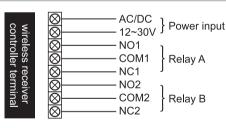
NOTE: This transmitter is used with the ADC-EB-602FD receiver, which can only connect to the B relay connection port. The relay output of the receiver, according to the dip switch of the transmitter.
