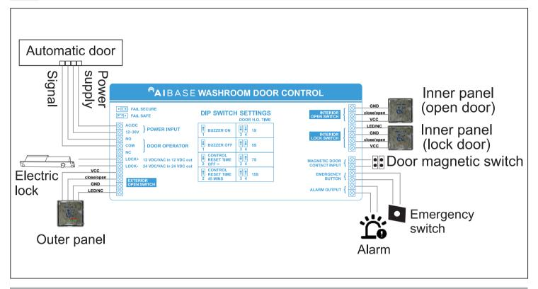
NOTE: 1, Controller power input is 12V power, also electric lock should be 12V; Or 24V for both.
