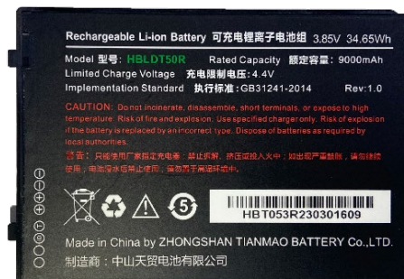
Figure 4-3 DT50P battery 9000mAh
