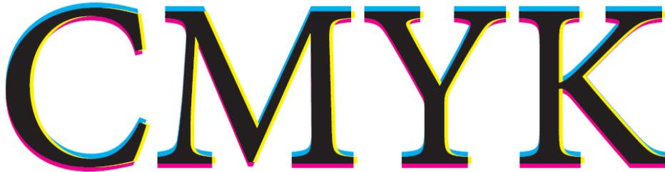
The image shows the word "CMYK" in a large, bold, serif font. Each letter is surrounded by a multi-colored halo or bleed-through effect, consisting of thin lines of cyan, magenta, and yellow. This illustrates the problem of misalignment during printing when using a CMYK black color that contains these three colors.
