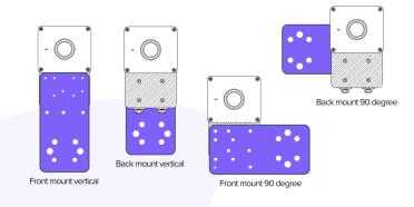
It's normal for the OV20i to become hot to touch when powered. For high temperature environments, use the front mounting points.
