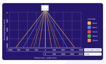
The camera has a 4:3 aspect ratio. Multiply the width by 0.75 to calculate the height.
