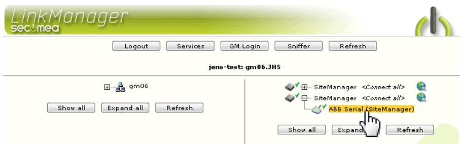
2. When connecting the agent, you should see some activity in the tray icon area, which is the auto configuring of a virtual serial port. If your SiteManager, and ABB PLC is correctly attached, you should also see the status of the agent become OK, and a few bytes of traffic:
