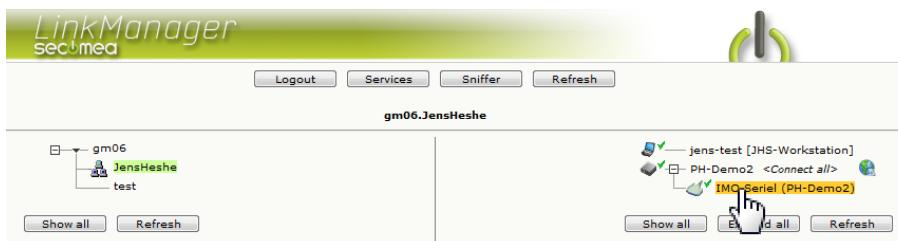
2. When connecting the agent, you should see some activity in the tray icon area, which is the auto configuring of a virtual serial port. If your SiteManager, and IMO PLC is correctly attached, you should also see the status of the agent become OK, and a few bytes of traffic:
