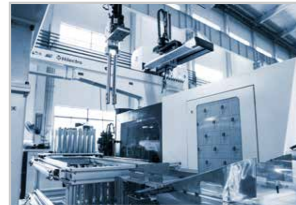
XTA Series High-Speed Servo Robot Integrated auxiliary machine automation Production case: automatic packing of knife, fork and spoon parts Production requirements: 16-cavity, 50 pc automatic packaging
