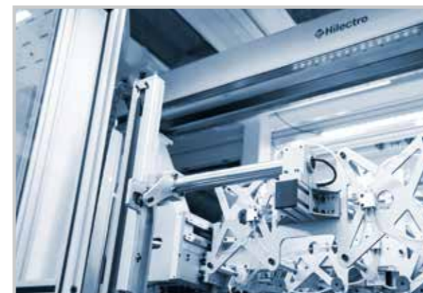
XTS Series Side Takeover with Labeling Integrated conveyor line Production case: milk cup with side takeout and labeling Production requirements: 8-cavity
