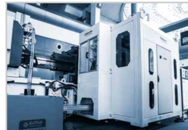
XTS Series Side Takeout with Mold Stack and Labeling Integrated conveyor line Production case: side takeout with mold stack and labeling of the container boxes Production requirements: 2 boxes + 2 caps
