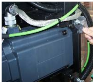
① Loosen adjusting screw nuts
