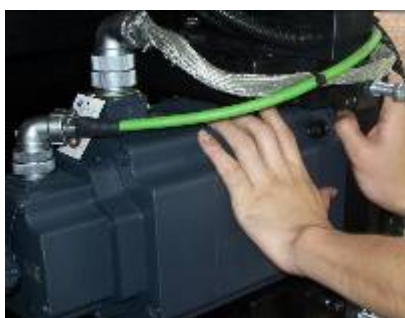
⑤ Push clamping motor to the machine. Loosen synchronous-belt
