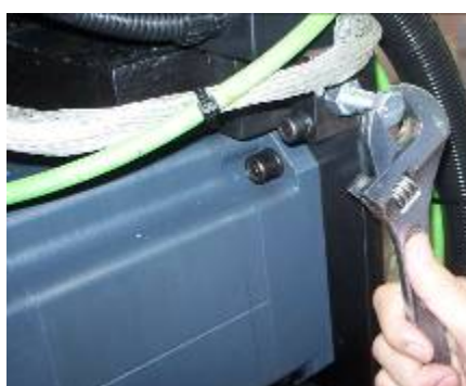
② Loosen tension adjusting bolts (2 pieces)
