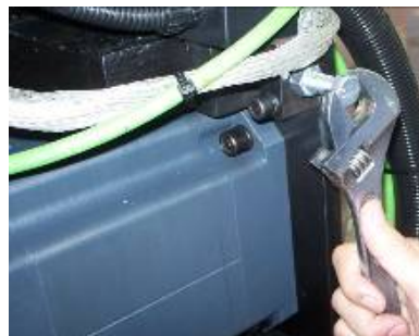
② Loosen tension adjusting bolts
