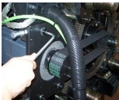
③ Loosen flange connection bolts
