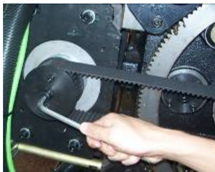
④ Screw off bolts (3 pieces), and take down the gear cover
