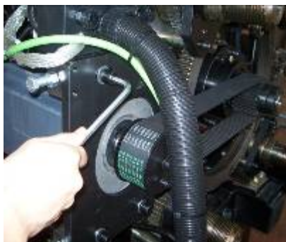
③ Loosen flange installation bolts (4 pieces)
