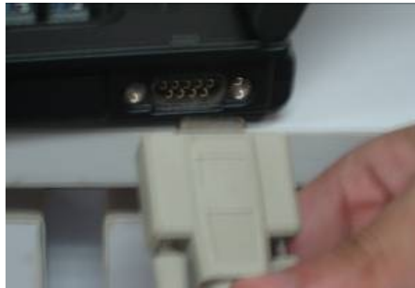
Fig2.2.3(3) Connect the serial port of a laptop with the other end of HSP5 line
