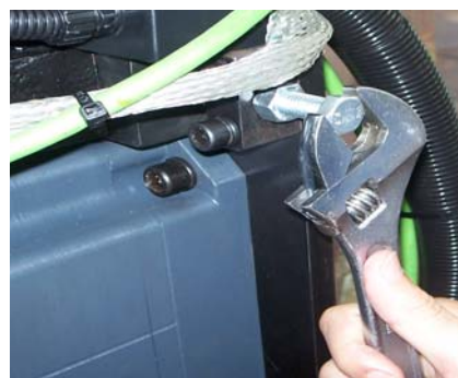
② Dismantle tension adjusting bolts (2 pieces)
