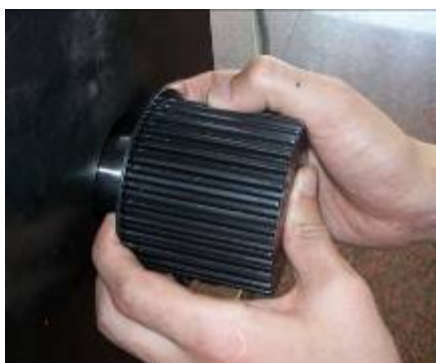
① Dismantle synchronous-belt with wheel
