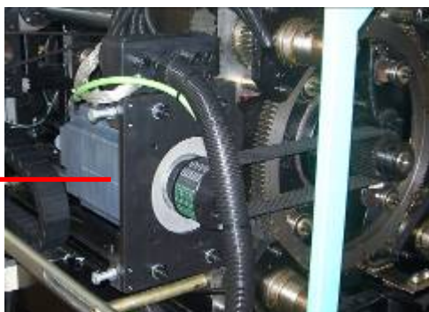
③ Strain the synchronous-belt by moving the motor outward (the arrow shows).
