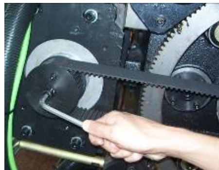
②Install bolts (3 pieces) and gear cover
