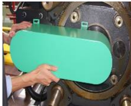
② Dismantle gear protection cover
