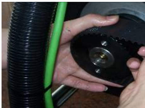
①Put a belt on one gear, then tighten the belt and put the belt on the other gear.
