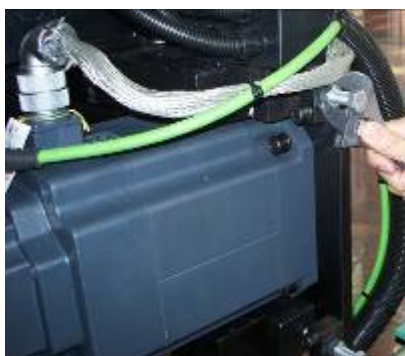
① Loosen adjusting nuts (2 pieces)
