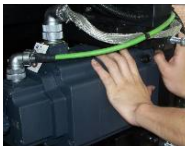
⑤ Push clamping motor to the machine to loosen synchronous-belt
