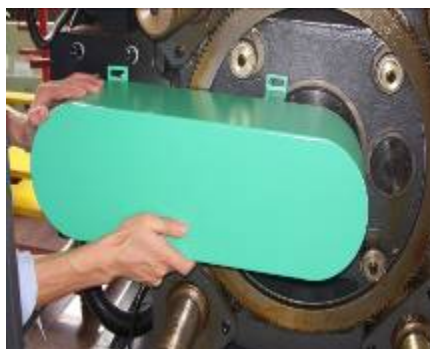
② Dismantle gear protection cover
