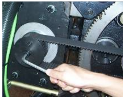
④ Loosen cover bolts remove gear cover
