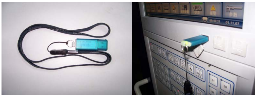
Fig 5.2.6(6) Connect the USB connector with a special U disk
