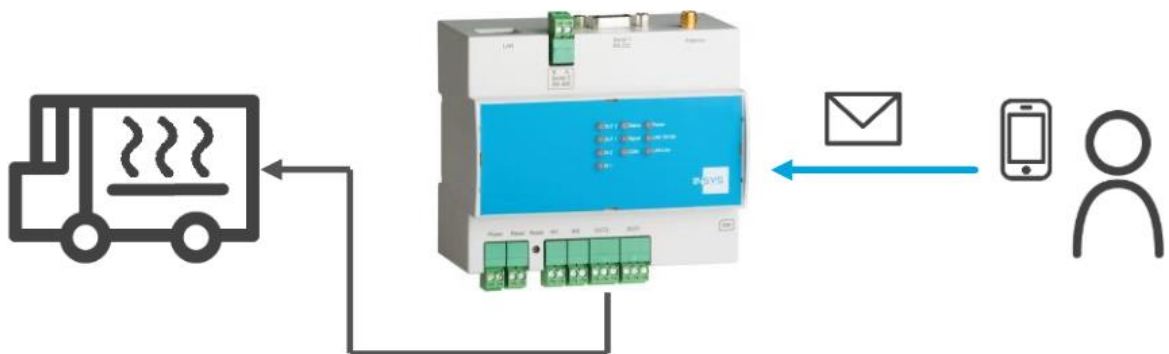
Figure 1: Switching an output via SMS – overview
