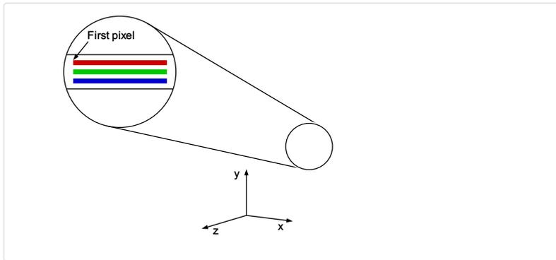
Alignment and orientation of the 10k sensor
