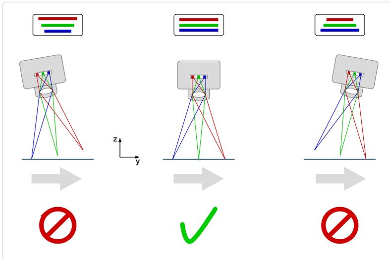
**Rotation around the transverse axis of the sensor**
